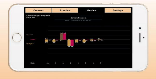
The **Metric** being displayed can be changed by double tapping the screen, the available metrics are Lateral Range, Vertical Range, Roll Range, Stroke Tempo and Acceleration Index. The **Page** (if more than 10 shots exist in the Session) being displayed may be changed by swiping the screen to the left or to the right. The **Session** being displayed may be changed by swiping the screen up or down.
